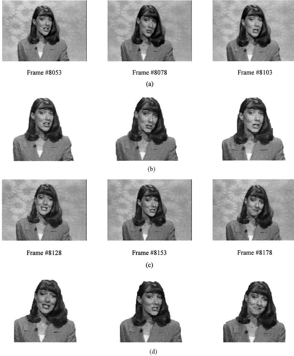
Fig. 10. Segmentation performance of the proposed adaptive neural-network architecture for several frames of the shot of Fig. 7 (first retraining phase). (a), (c) The original frames. (b), (d) The respective segmentation mask of the foreground object.
